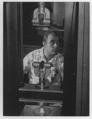
PROOF TESTING of components is performed by Richard Bohannon, 1611, who operates device to "squeeze" small aluminum container with predetermined pressures. Tests like these give scientists an idea of effects of stress and strain on various weapons parts.
